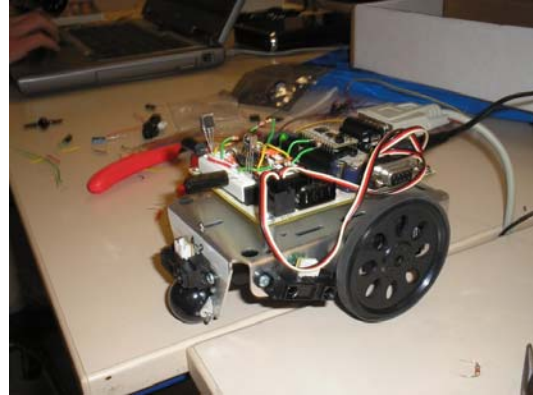
Figure 5: Second prototype robot with IR sensors
