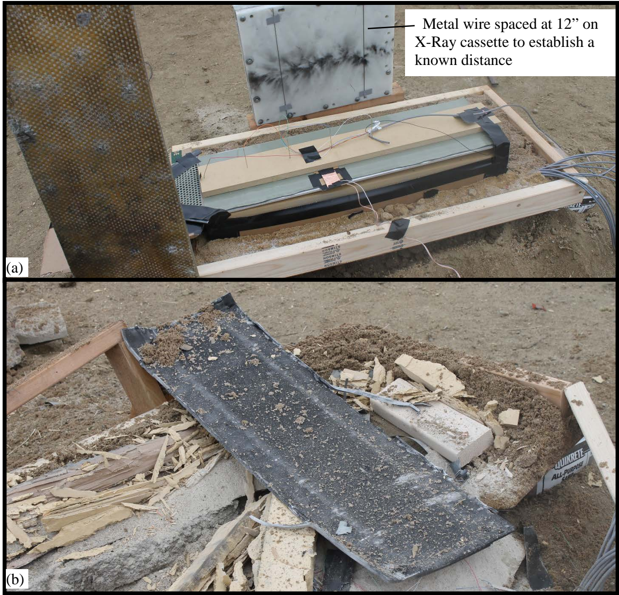
Figure 3-19: 1.5° test. a) Test before detonation. b) Post-welding result.
