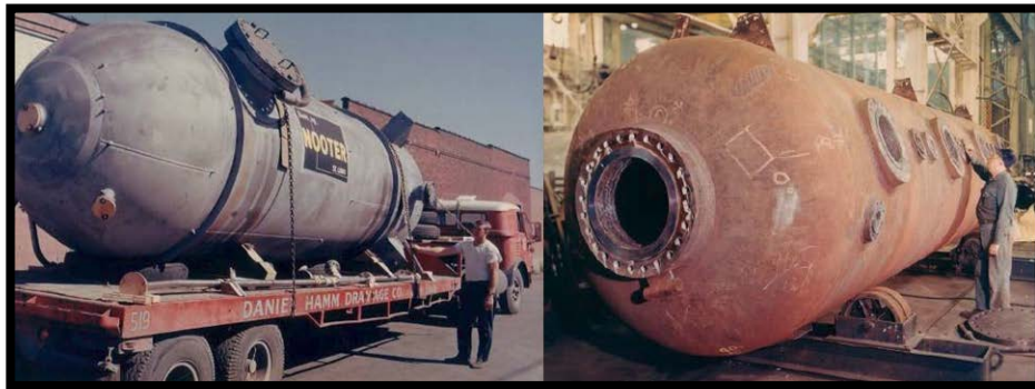
Figure 2-10: Early DuPont cladding products. Left: a terephthalic reactor ready for delivery. Right: a metal leaching autoclave in production. Images courtesy of John Banker, of Clad Metal Consulting, an early DuPont employee. [36]
