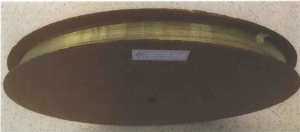
Figure 4.3. Spool of 2 mm diameter BCF-91A wavelength shifting fiber manufactured by Saint-Gobain Ceramics & Plastics, Inc.
