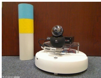
Figure 4: Robot node implemented with an iRobot Create.
