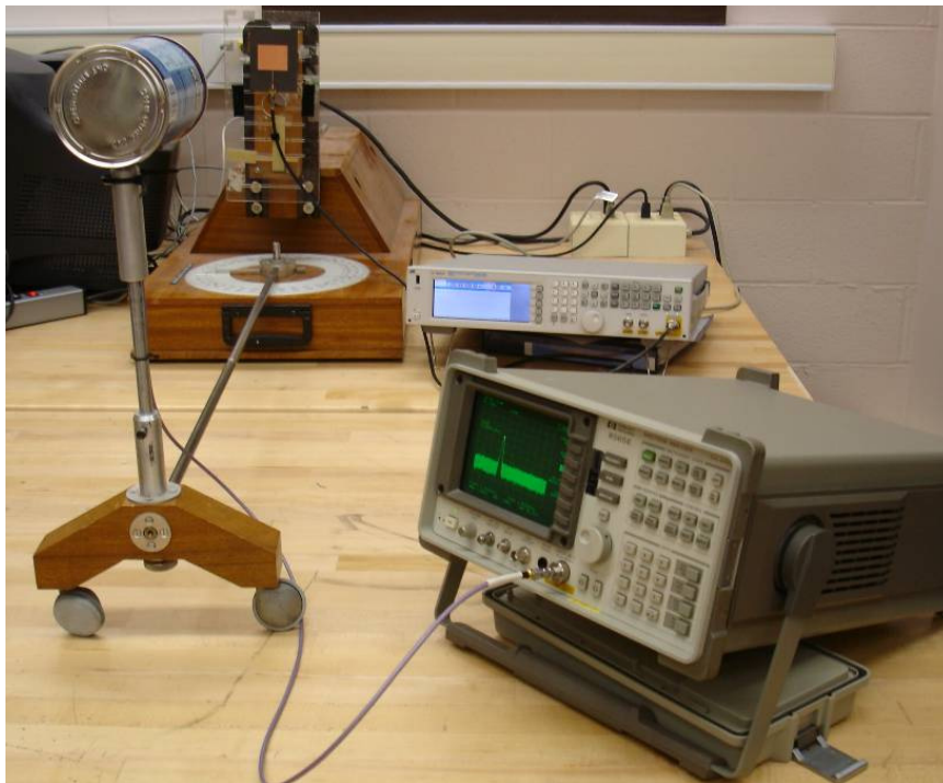
Figure 4.14. Experimental apparatus for measurement of radiation patterns.
