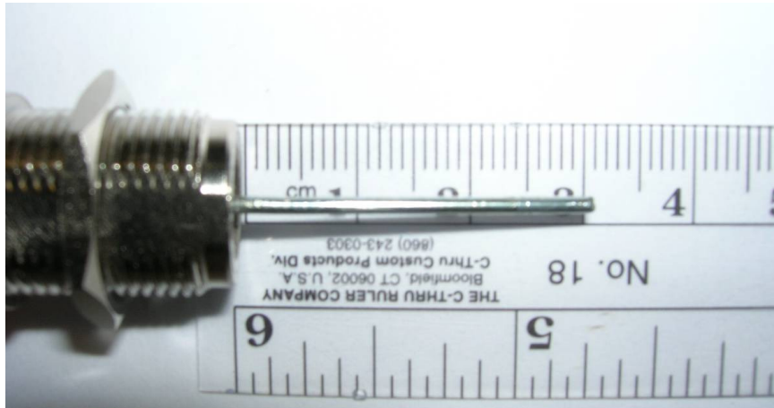
Figure 4.17. \lambda/4 wire antenna, soldered into 50 \Omega female N-type bulkhead connector.
