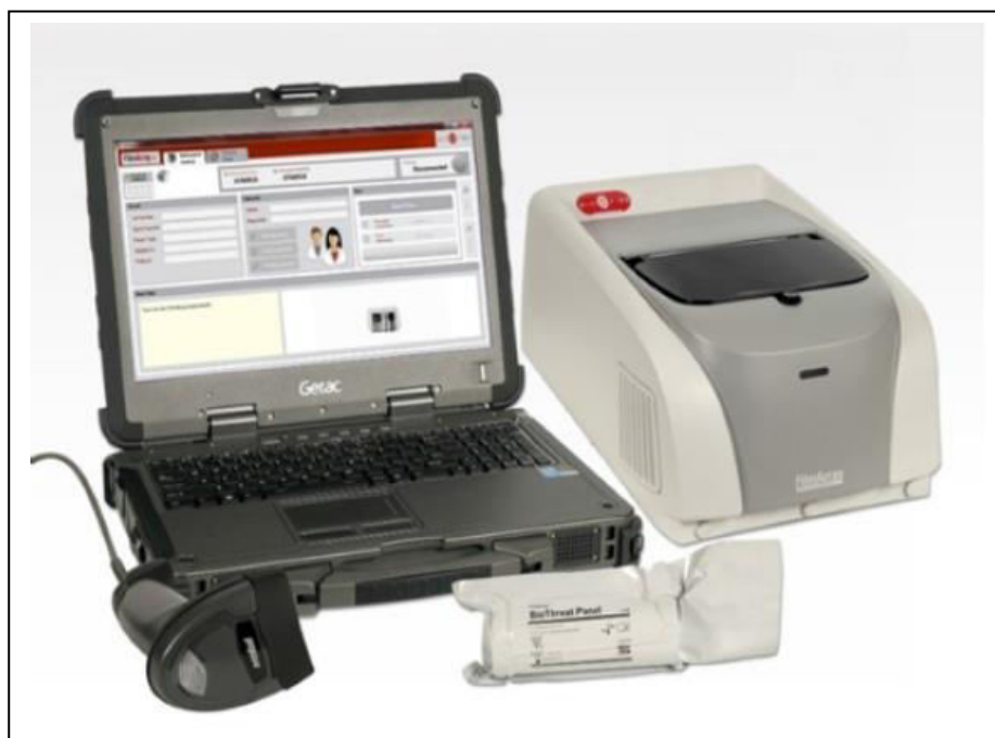
Figure 3: The Next Generation Diagnostics System Increment 1 (NGDS-1), also known as the Bio Fire Film Array® 2.0. This figure was extracted from Next Generation Diagnostics System, Increment 1 Fact Sheet, 7/27/2017. Point of Contact: Chemical, Biological, Radiological, & Nuclear Information Resource Center (CBRN IRC), CBRN.IRC@mail.mil , Toll Free: 18008314408, Commercial: (309) 7827349, DSN: 7937349, Fax: (309) 7821919.
