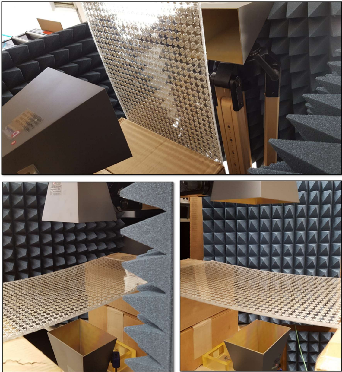
Figure 5.34. Free-space measurement setup of finite FSS array encapsulated in Sylgard-527.
