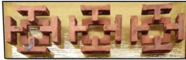
Figure 5.3. Example 3D FSS unit cells coated with \sim 5\mu\text{m} of copper using an electroless copper solution.
