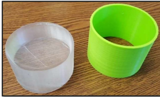
Figure 5.6. S-Band dielectric cylindrical cavity (left) formed using a 3D printed PLA cylindrical shell (right).
