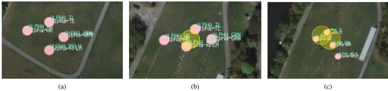
Fig. 5: Examples of misshapen wedge formations and robot collisions.
