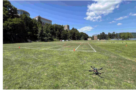
Fig. 7. Flight test field: 16 orange traffic cones simulate landmines, with a drone at the bottom right
